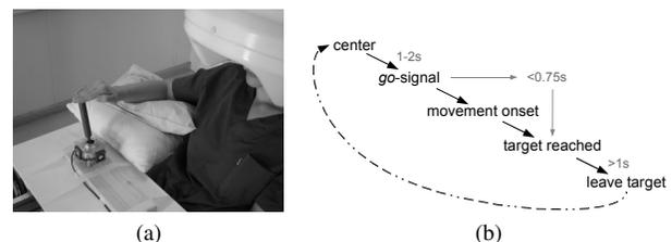
Fig. 1. (a) Experimental setup. (b) Sequence of one trial along with time constraints.
