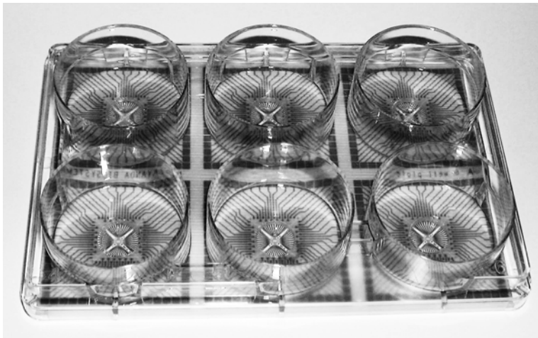
Figure 10-15. 8-well multiple MEA recording device. This type of developments is intended either for simultaneous recording from cell cultures or for acute slices (by courtesy of Ayanda Biosystems, Lausanne, CH).
